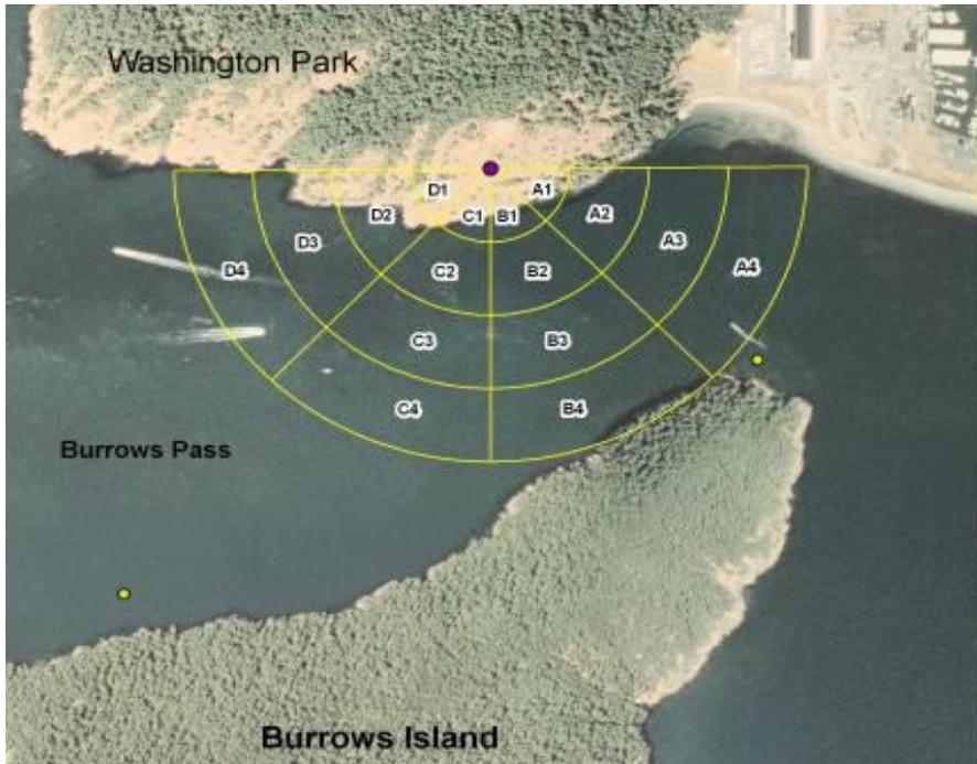
We have tested additional aids, such as reticular binoculars and theodolite apps, and have selected a draped grid transparency that the observer can hold in front of them to check the porpoise location. This location tool will be used for future observations, and we are developing methods to test its accuracy. An example of the grid this tool creates is shown below.
